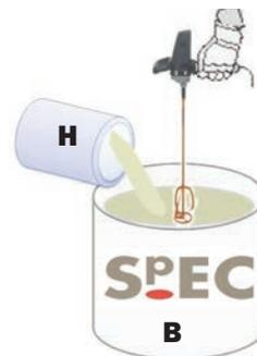
Empty the entire contents of the curing agent into the base component. To ensure that all material is extracted, the insides of the tins should be scraped. The curing agent and the base component should
